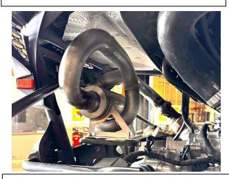
4. Wipe the exhaust clean using a degreaser or rubbing alcohol to remove all fingerprints prior to starting the vehicle. Double check all hardware after your first 20 minutes of riding to be sure everything is still tight.
