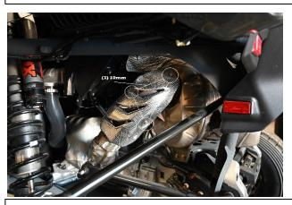
2. To remove the factory muffler, you'll need to remove the heatshield covering the head pipe which is held on by 3 10mm bolts. Then, remove the 4 springs holding on the exhaust head pipe and the 4 bolts holding the muffler to the frame of the vehicle located beneath the muffler assembly. You will be reusing the stock bolts.
