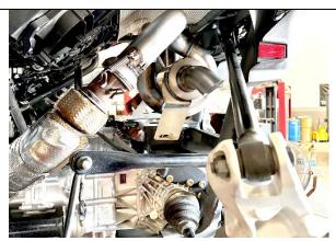
3. Finally, install muffler assembly #A by fishing it through the passenger side wheel well. (BE CAUTIOUS AND PATIENT WHEN FISHING IT THROUGH AS IT IS A TIGHT FIT.) Once in place reinstall the 4 bolts that secure the muffler loosely then install all 4 springs to the head pipe, once springs are installed go back and tighten the 4 bolts securing the muffler.
